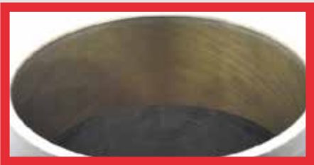
LINERS Liners are still in excellent condition, demonstrating minimal wear with cross hatching marks clearly intact.
